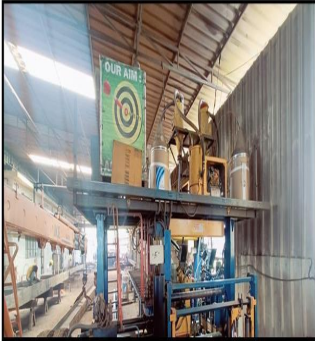
Photo 5: submerged arc welding machine (SAW)
